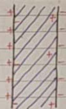
Fig-1 Schematic illustration of charges induced at the surface of a dielectric.
