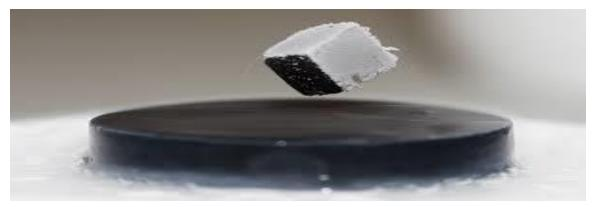
A sufficiently strong magnetic field will destroy superconductivity.
